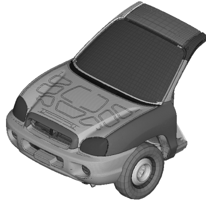
Fig. 1 Finite element model of a sedan
