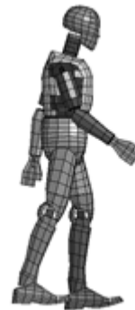
Fig. 3 Finite element model of a pedestrian dummy
