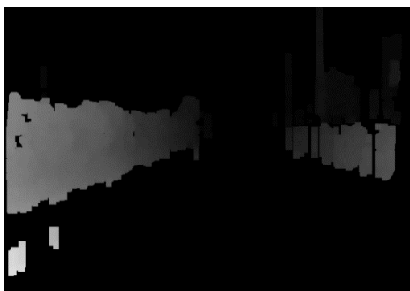
Fig. 3. Result of road surface removal using U-disparity map
