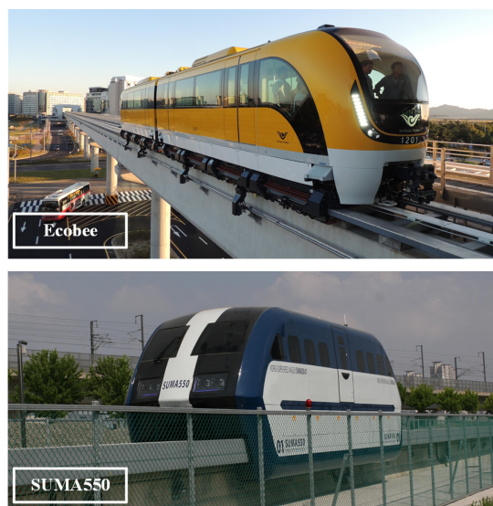
Fig. 1. Maglev Train in Korea. ECOBEE (110 km/h urban class); SUMA550 (550 km/h high-speed class)
