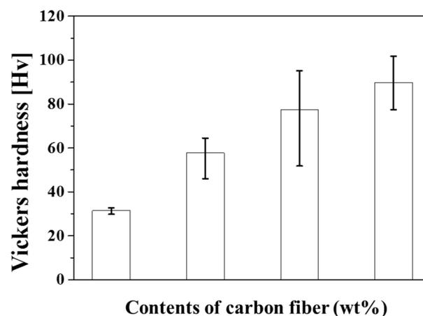
Fig. 3. Vickers hardness measurements of each carbon fiber content.
