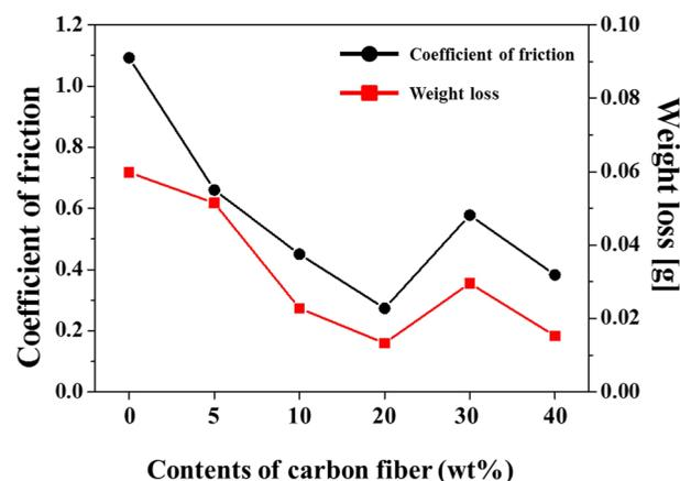
Fig. 4. The average coefficient of friction and weight loss of each carbon fiber content.
