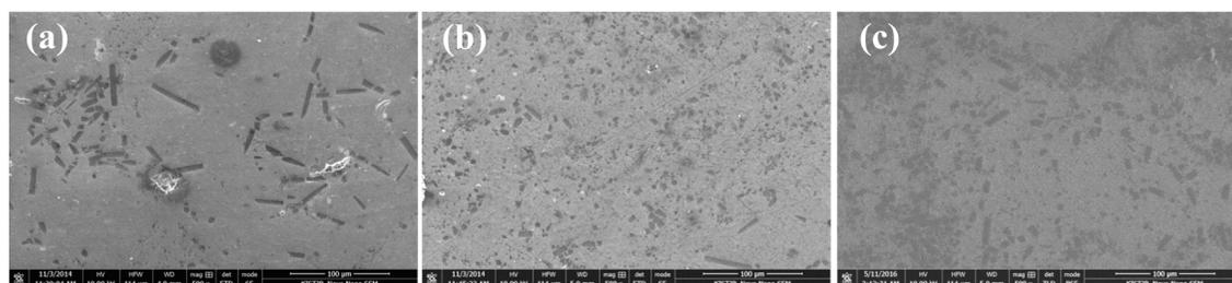
Fig. 2. Scanning electron microscopy images of the sintered surface displaying the distribution of carbon fibers: (a) 5 wt%, (b) 10 wt%, (c) 20 wt%.
