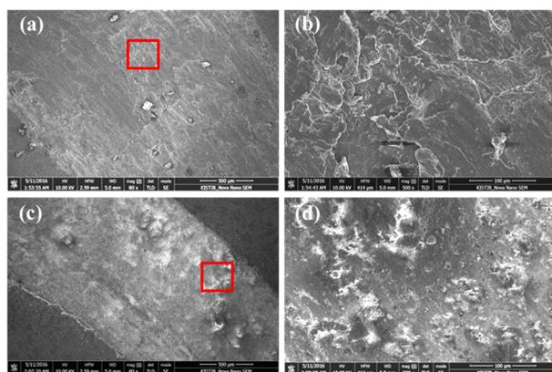
**Fig. 5.** Scanning electron microscopy images analyzing the surface of (a, b) the pure Al and (c, d) the 20 wt% after the wear test. (b, d) represent higher magnifications for (a) and (c), respectively (marked with red squares).
