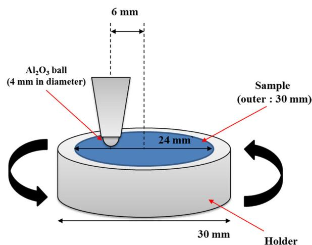
Fig. 1. Schematic illustrating the friction test.
