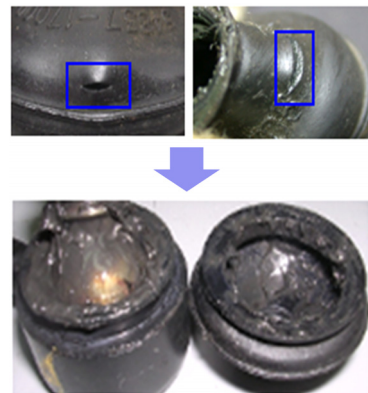
Fig. 7 Water ingress by dust cover damage
