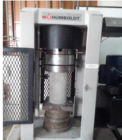
FIGURE V Compressive Strength Testing of Concrete
