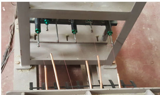
Photo 4. Connection of high strength composite fiber installed on geogrid in pullout box
