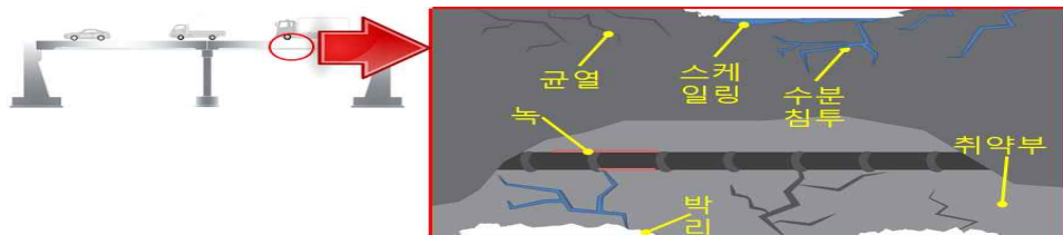
Fig. 1. Concrete deterioration phenomenon
