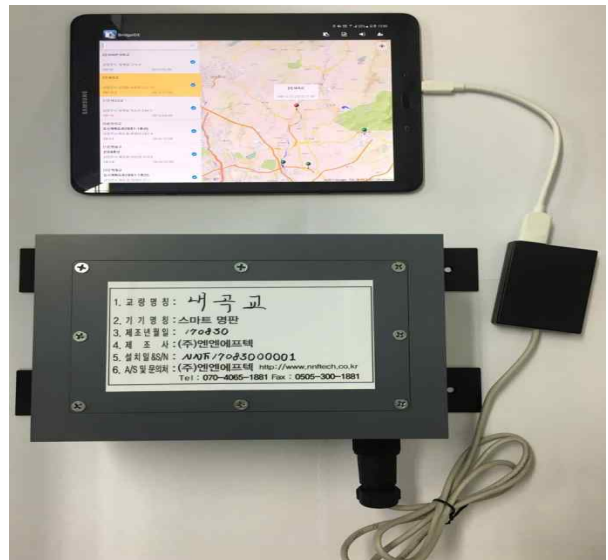
Fig. 13. Integration Test of Smart Nameplate through Bridge Maintenance Mobile Program and Reader
