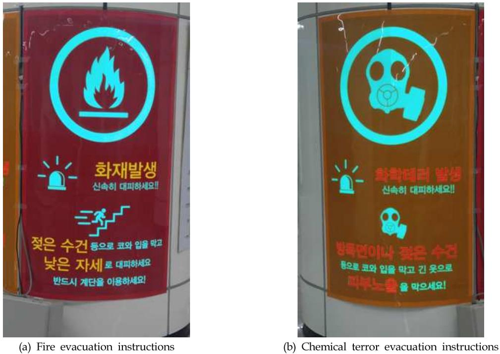
Fig. 18. Circular column-mounted EL display module
