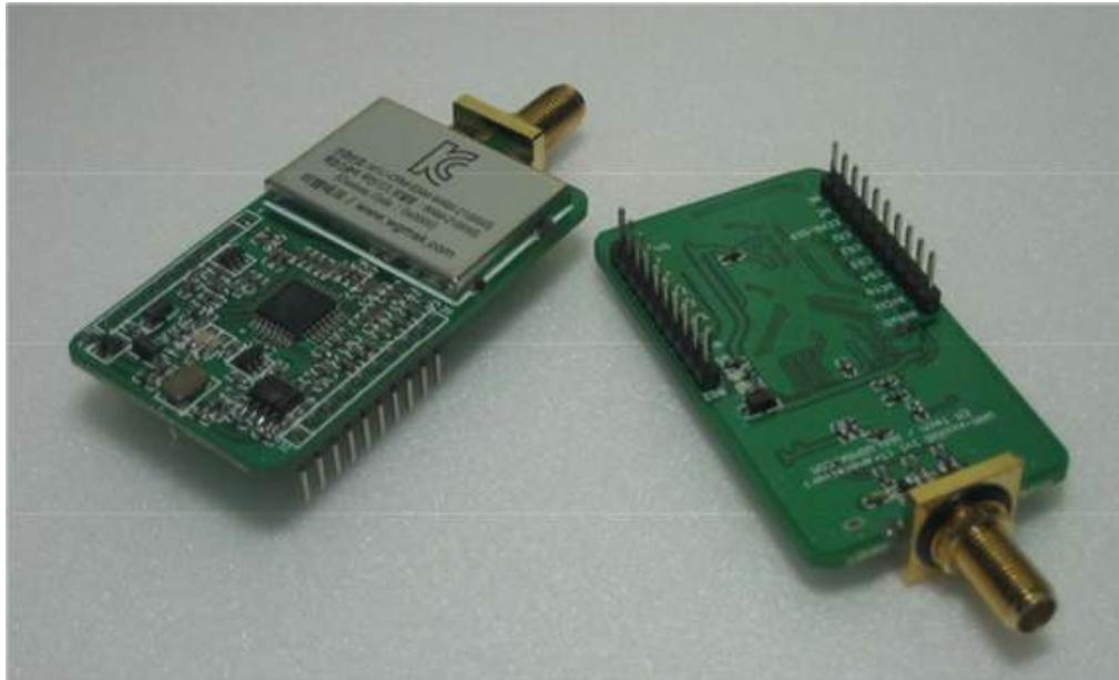
Fig.14. EL display control communication module
