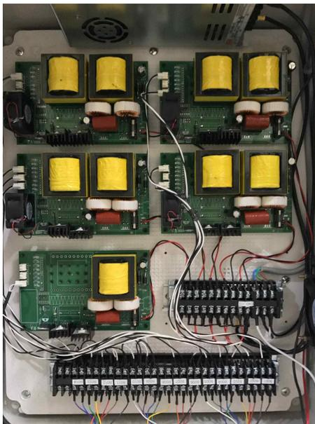
(a) Large capacity EL panel Inverter layout
