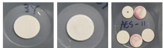
(a) ZrO_2(3Y) (b) ZrO_2(8Y) (c) Al_2O_3 Fig. 9 Photograph of sintered ceramic specimens
