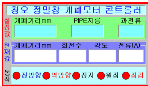
Fig. 1. Display screen of the window motor.
