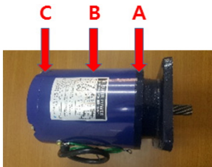
Fig. 2. Locations of the vibration measurement on the motor.
