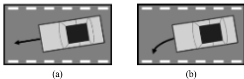
Fig. 2. Straight road section (a) Zero steering (b) Constant steering
