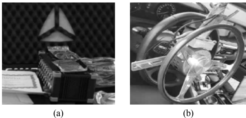
Fig. 6. Test measuring device (a) DAQ (b) Steering wheel sensor
