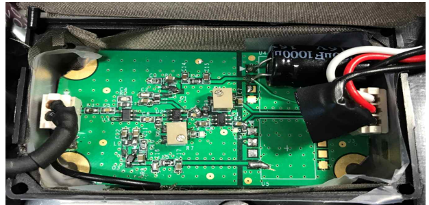
Fig. 3. PCB of Charge Sensitive Amp, Pulse Shaping Amp, Discriminator
