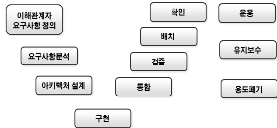
[Figure 4] Systems Engineering Development Process
