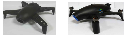
(a) Initial Design (b) After Design Change Fig 14. Before Change & After Change of Airframe Shape
