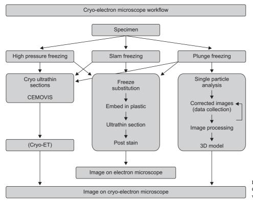
Fig. 1. Cryo-electron microscope workflow. CEMOVIS, cryo-electron microscopy of vitreous sections; ET, electron tomography.
