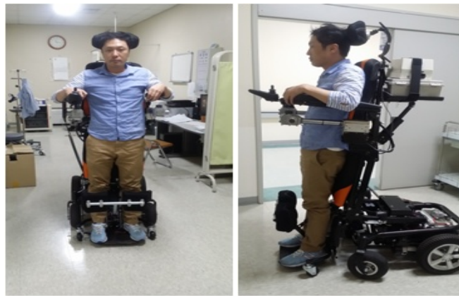
Fig. 12 . The implementation result of standing of the upper/lower limb rehabilitation wheelchair vehicle system
