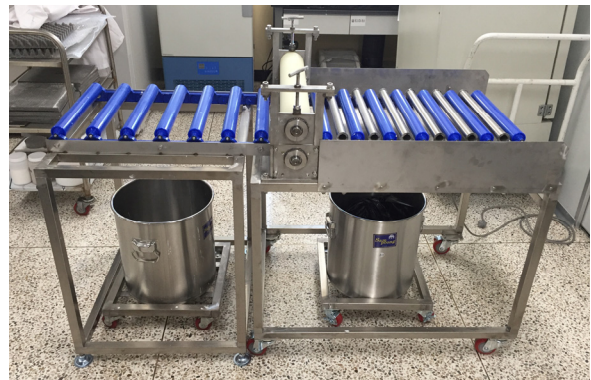
Fig. 2. Photograph of the rolling equipment for manufacturing the organic-inorganic hybrid materials
