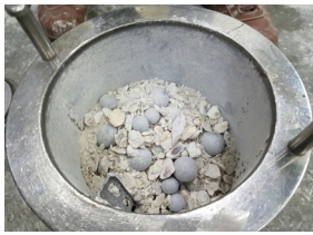
Fig. 16. Crushing result of ball mill
