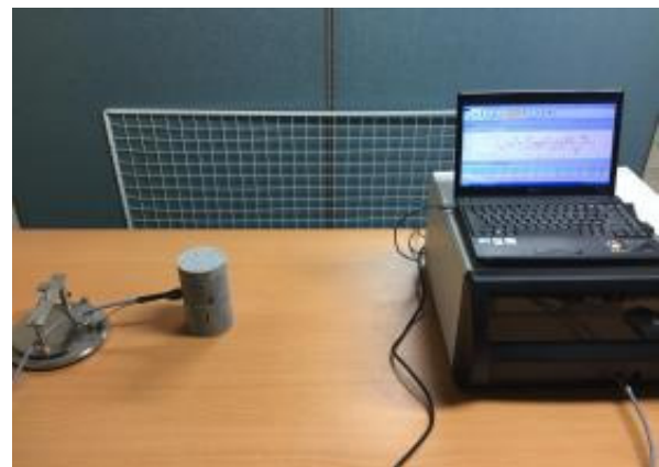
Fig. 6. Measurement of thermal conductivity
