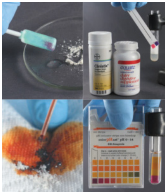
Fig. 1. Preliminary detection method for suspicious materials; protein, saccharide, pH and starch (clockwise from upper left) [8]
