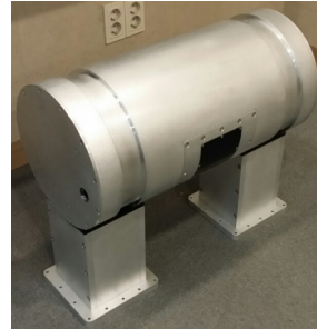
Fig. 11. Aluminum cylinder simulating a missile.
