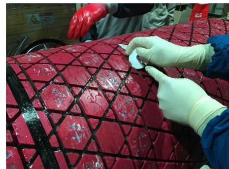
Fig. 2. Compression process of intersection points
