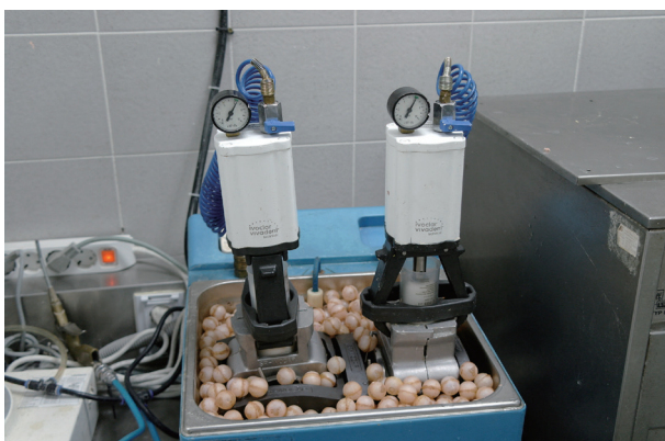
Fig. 8. Polymerization of denture using SR Ivocap system. Injection pressure was 6 bar and polymerization time was 35 minutes in 100°C water.
