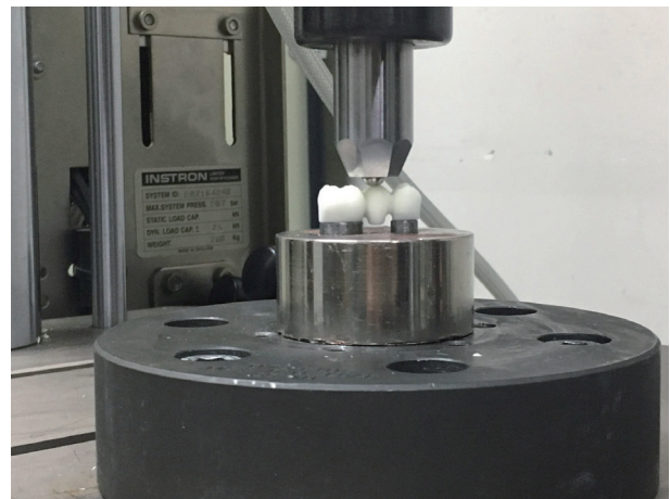
Fig. 3. Flexural strength test of specimen with Universal testing machine.
