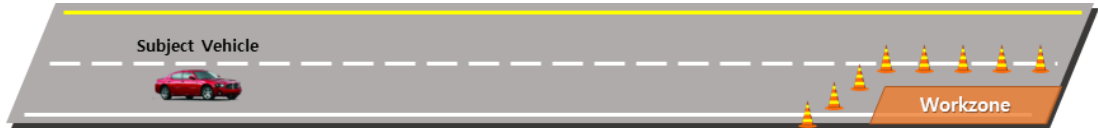
(c) Scenario 3 : No traffic sign installation in work zone
