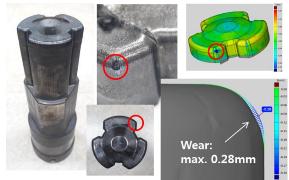
Fig.13 Tool wear of punch for tripod-housing
