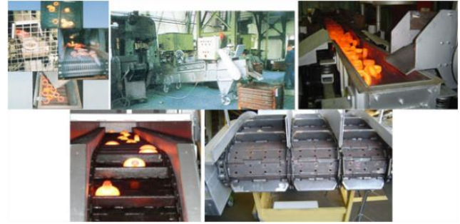
Fig. 2 Transfer system for controlled cooling following forging press
