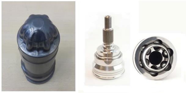
Fig.14 Tool wear of punch for BJ-housing
