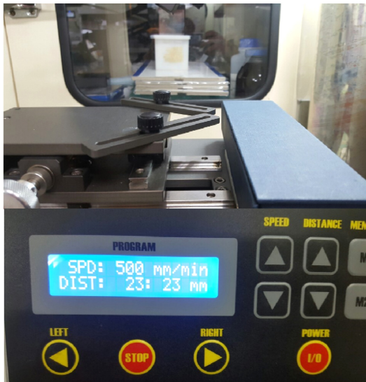
Fig. 7. Photograph of bending measurement tester of protective films.
