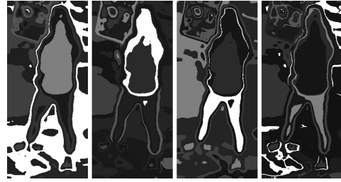
Fig. 3. K-means algorithm results (from the left K=11,12,13,14)
