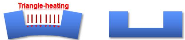
(a) Global distortion and triangle heating (b) After correction
