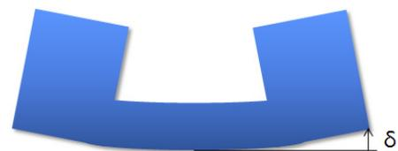
Fig. 5 Schematic reverse setting shape of block
