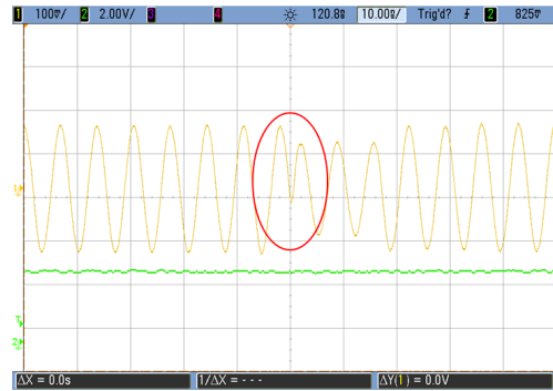
(c) FMCW 180° 위상변조 측정 (c) Measured Bi-phase Modulated FMCW
