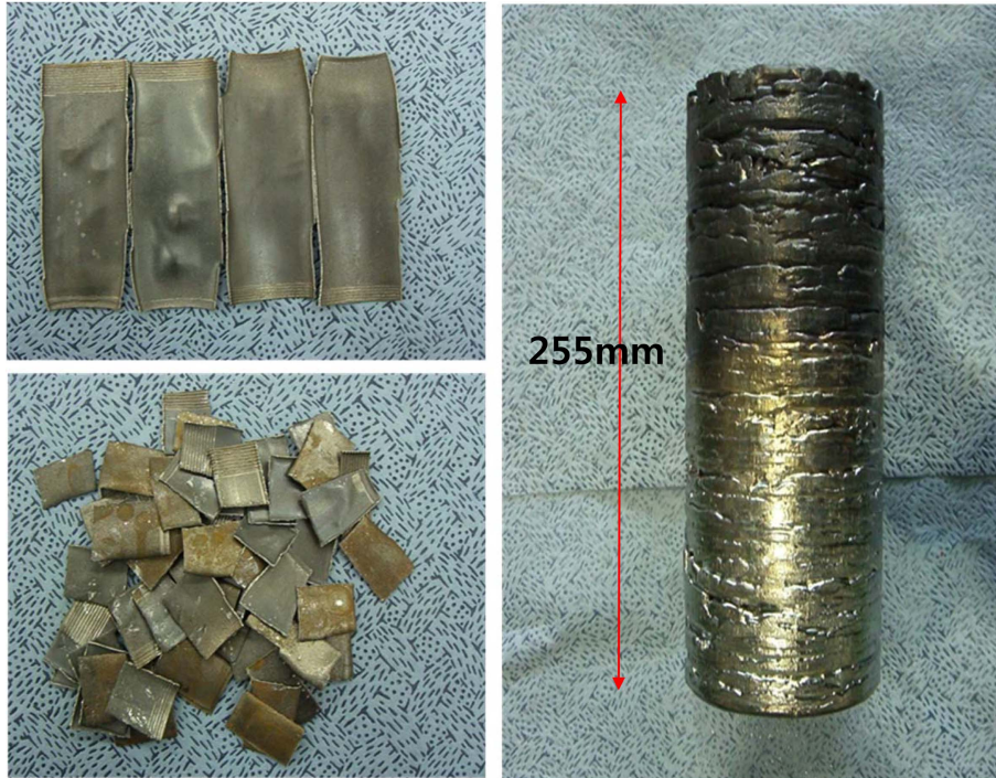
Fig. 10. Photograph showing the zirconium alloy ingot produced by plasma arc remelting process using Zr alloy of old scraps. (Ar gas atmosphere)
