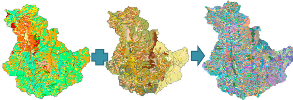
Fig. 3. Process of making HRU distribution map using land use map and soil map
