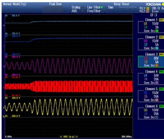
Fig. 19. Step response in capacitor voltages of HSF1 and LSFI along with HSF1, LSFI and load voltage waveform.
