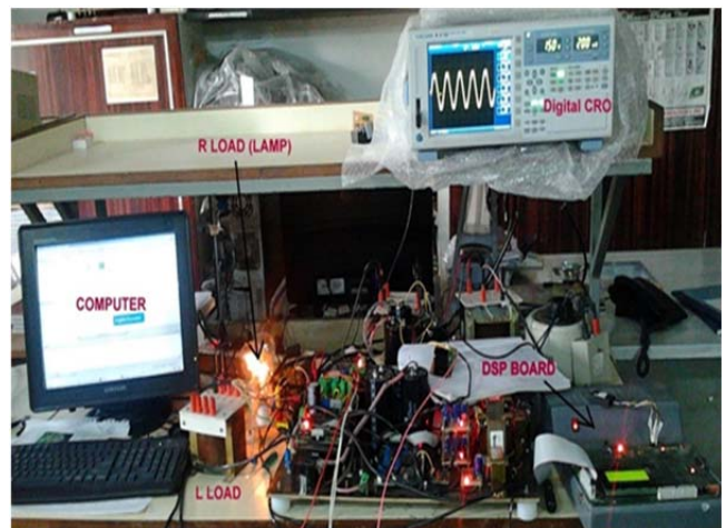
Fig. 17. (a) Schematic diagram for the hardware Setup of the proposed inverter (15 Levels), (b) hardware Setup of the proposed inverter.
