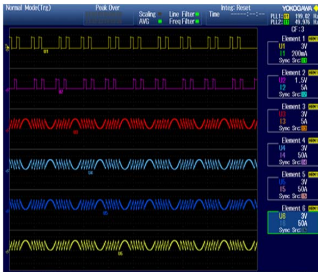
Fig. 20. Switching pulses and reference waveforms (a) Auxiliary switch 1 (b) Auxiliary switch 2 (c, d, e and f) Reference waveforms of the HSF1 [Without capacitor voltage balancing].
