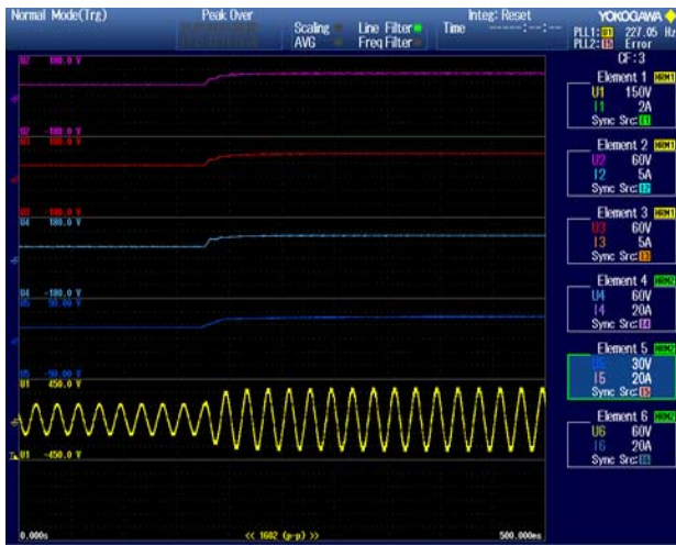
Fig. 18. Step response in Capacitor voltages of LSFI along with load voltage for a 7-level inverter without filter.
