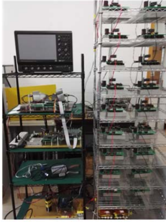
Fig. 9. Photo of a single-phase MMC prototype.
