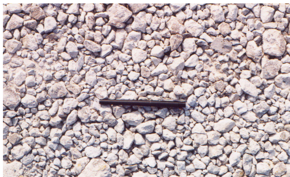
Fig. 5 Rubblized Concrete by Resonant Frequency Breaker
