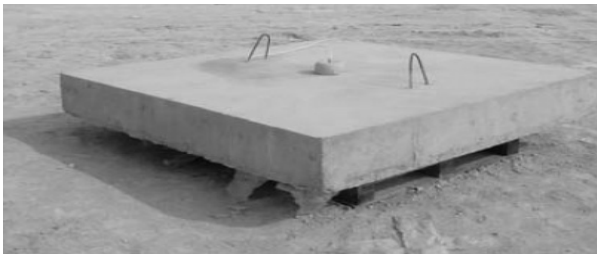
Fig. 3. Explosion Experiment Model of RC Slab
