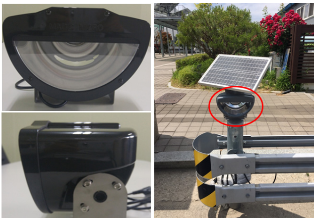
Fig. 13. Manufactured freeform reflector and application in road.
