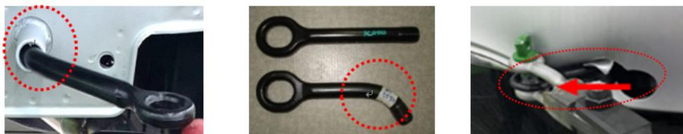
Fig. 3 Example of Towing hook deformation
