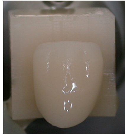
Fig. 2. Incisor crown milled in a 4 shades block.
