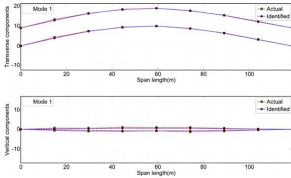
그림 4 Comparison of actual mode shapes and the identified system mode shapes for mode 1. (Mustafa, Debnath et al. 2015)
