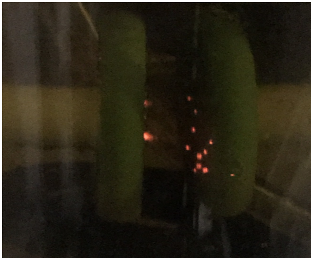
Fig. 8. Photograph of the corona discharge observed on the electrode surfaces.
