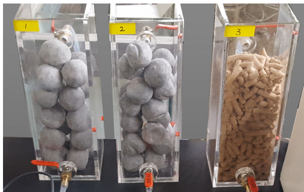
Fig. 1. Photographs of lime-based granular alkaline materials (left: Material_1, center: Material_2, and right: Material_3).
