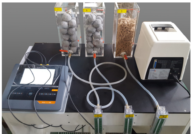
Fig. 2. Experimental equipment of column test for elution characteristics.
