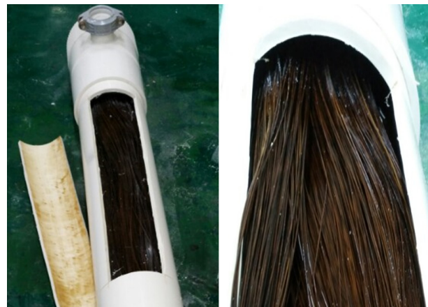
Fig. 12. Membrane module of contaminated by Manganese.
