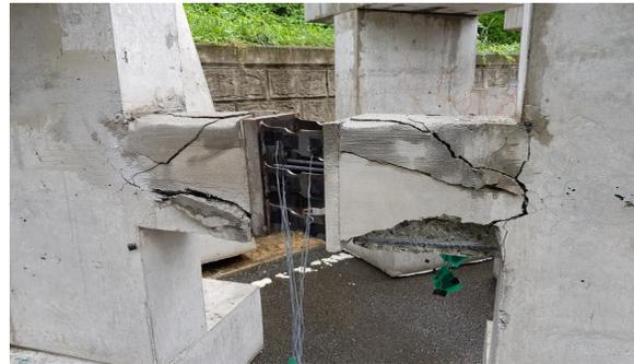
(a) SD specimen after testing
