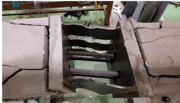
(b) Damper deformation of SD specimen
