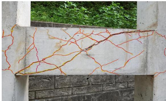
(a) Coupling beam of RC specimen
