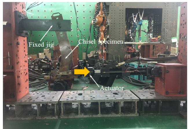
Figure 10. Chisel fatigue test setup.
