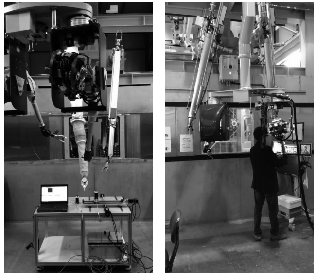
Fig. 2. Physical mock up for actual testing of remote procedures.
