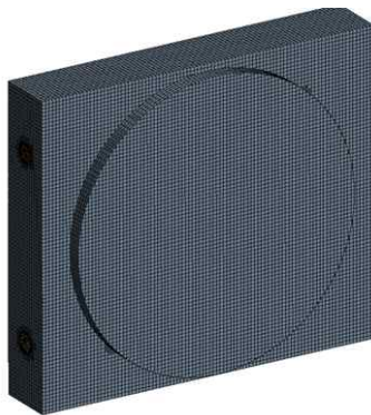
Trimmed mesh : 186,659 개 (b) Zigzag channel type
