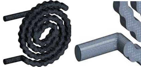
Polyhedral mesh : 658,307 개 (b) Zigzag channel type
