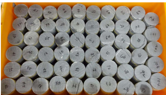
Fig. 3. Core samples from Danyang limestone after compressive experiment.
